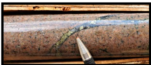
Plate 36: Late quartz+calcite vein utilizes and replaces magnetite with blebs of pyrite+chalcopyrite within OCP altered (quartz) monzonite @23.80m. Sample# 42537 containing 0.14% Cu, 0.04g/t Au, 0.28g/t Ag and 6.98ppm Mo over 1.00m.
