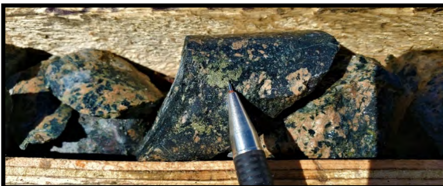
Plate 50: Coarse grained blebs of chalcopyrite within 10cm magnetite+chlorite vein breccia proximal to chloritic shear @240.90m. Sample # 42476 containing pyrite±chalcopyrite - 96.77m. Sample # 42365 containing 0.13% Cu, 0.03g/t Au, 0.12g/t Ag and 108.00ppm Mo over 0.60m.
