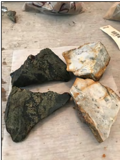
Plate 2: Sample #3261 (left) is a float sample taken below a chloritic shear zone containing semi-massive pyrite replacing magnetite. Sample #3264 (right) is a 7cm quartz-calcite breccia within an east-west trending fault zone containing trace disseminated pyrite±chalcopyrite.
