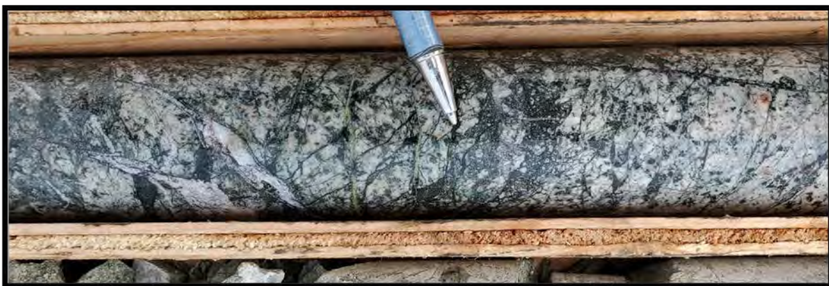
Plate 45: Sheeted and vein brecciated actinolite cut by epidote±quartz and late dilational calcite veins within pervasive, texturally destructive SCA within medium to coarse grained diorite @35.20 meters. Trace sulphides noted within the actinolite likely associated with epidote and quartz.
