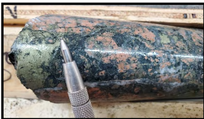
Plate 27: Coarse, blebby chalcopyrite and lessor pyrite proximal to late calcite vein that cuts chloritic shear breccia infilled with magnetite (K-feldspar selvage) and silica. Host is diorite @59.00m just above shear zone. Sample# 60473 containing 0.15% Cu, 0.05g/t Au, 0.37g/t Ag and 1.87ppm Mo over 1.00m.
