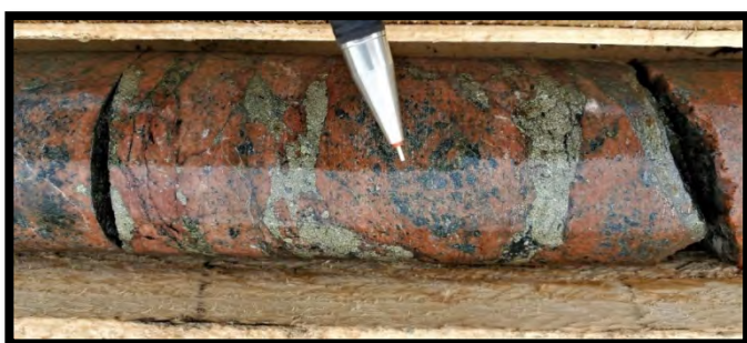
Plate 33: Localized OCP alteration related to magnetite veining within (quartz) monzonite shows granular pyrite±chalcopyrite replacing magnetite @121.00m. Sample# 43070 containing 0.35% Cu, 0.07g/t Au, 1.66g/t Ag and 6.72ppm Mo over 1.00 meters.
