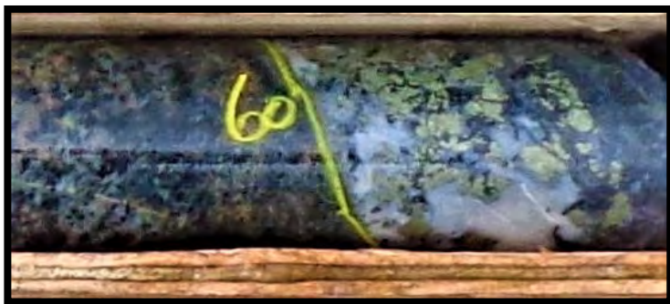
Plate 11: Isolated 10cm quartz-calcite±magnetite vein @60.33m contains coarse grained blebs of chalcopyrite+pyrite. Sample# 76109 containing 0.64% Cu, 0.026g/t Au, 1.20g/t Ag and 1.69ppm Mo over 1.00m.
