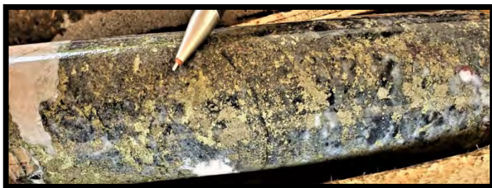
Plate 37: Blebs of pyrite+chalcopyrite within silica brecciated magnetite vein containing late coarse calcite proximal to increased mineralization @72.50m. Sample# 42580 containing 3.42% Cu, 0.75g/t Au, 7.03g/t Ag and 1.13ppm Mo over 0.50m.
