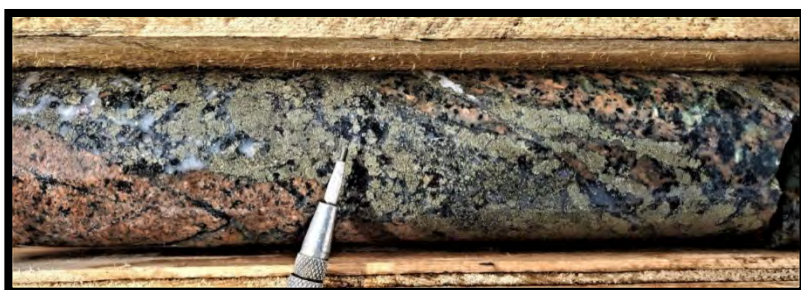
Plate 38: Blebs of pyrite+chalcopyrite within silica brecciated magnetite vein containing late coarse calcite proximal to increased mineralization @123.60m. Sample# 42626 containing 0.56% Cu, 0.14g/t Au, 0.85g/t Ag and 2.10ppm Mo over 0.60m.
