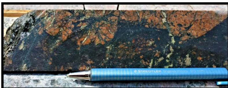
Plate 20: Semi-massive magnetite breccia with associated K-feldspar alteration of (quartz) monzonite and late pyrite+chalcopyrite fractures, blebs and disseminations cutting and replacing magnetite @165.80m. Sample #76505 containing 0.34%Cu, 0.09g/t Au and 0.97g/t Ag and 3.47ppm Mo over 0.68m.
