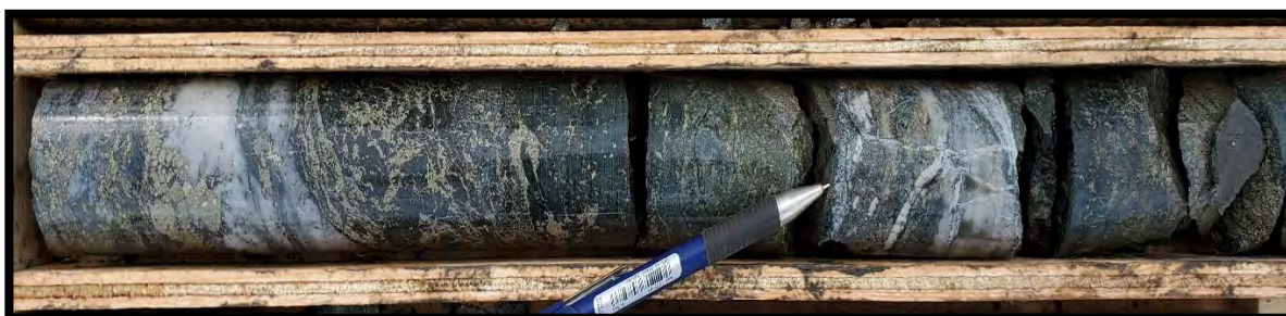
Plate 23: Section of lower mineralization zone (40cm) within a moderately silicified and quartz veined chloritic shear containing semi-massive magnetite cut by quartz and sulphides, the latter replacing magnetite. Sample# 41340 containing 1.84% Cu, 0.45g/t Au, 9.49g/t Ag, and 73.70ppm Mo over 0.64 meters.
