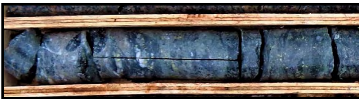
Plate 13: Polyolithic breccia (30cm) @110.50m with chloritic matrix containing interstitial and blebby quartz-calcite-chalcopyrite-pyrite. Sample# 76161 containing 0.57% Cu, 0.29g/t Au, 3.94g/t Ag and 4.52ppm Mo over 1.00m.
