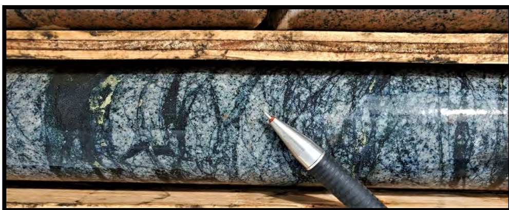
Plate 25: Semi-stockwork to sheeted veins and fractures of magnetite and later actinolite with associated pervasive albite alteration and disseminated to blebby pyrite and chalcopyrite replacing magnetite @ 104.7m. Sample# 41385 containing 0.17% Cu, 0.04g/t Au, 0.50g/t Ag and 7.43ppm Mo over 0.46 meters.
