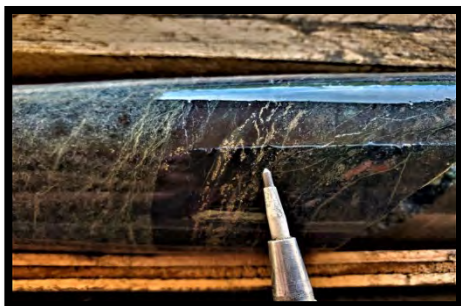
Plate 32: Magnetite vein within isolated, moderately silicified chloritic shear both cut by late, hairline fractures of quartz-epidote-pyrite and lesser calcite @25.26m.
