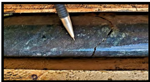
Plate 35: Barren, semi-massive magnetite veining with interstitial secondary chlorite, actinolite, calcite and quartz @15.40m.
